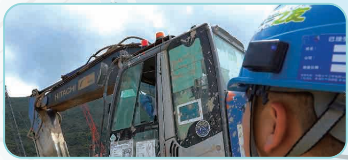
當工友進入機械操作範圍，智能安全帽便會發出聲響及震動 When worker enters to the range of machinery operations, smart helmet will emit sound and vibration
